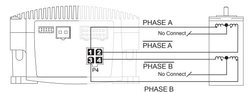
Figure 2.3.5: 6 Lead Half Coil (Higher Speed) Motor Connections
